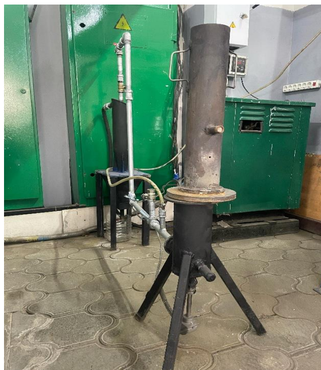
1 – the agglomeration bowl; 2 – dust collection unit; 3 – slide gate; 4 - storage bunker; 5 – vacuum chamber; 6 – thermocouple.
