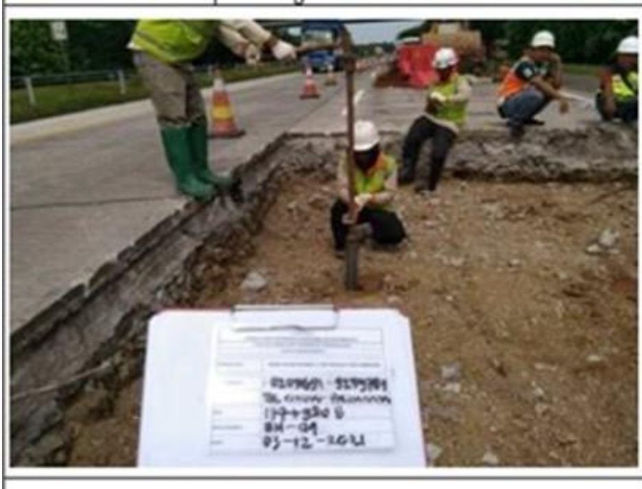
Figure 8. UDS sampling using hand auger.
