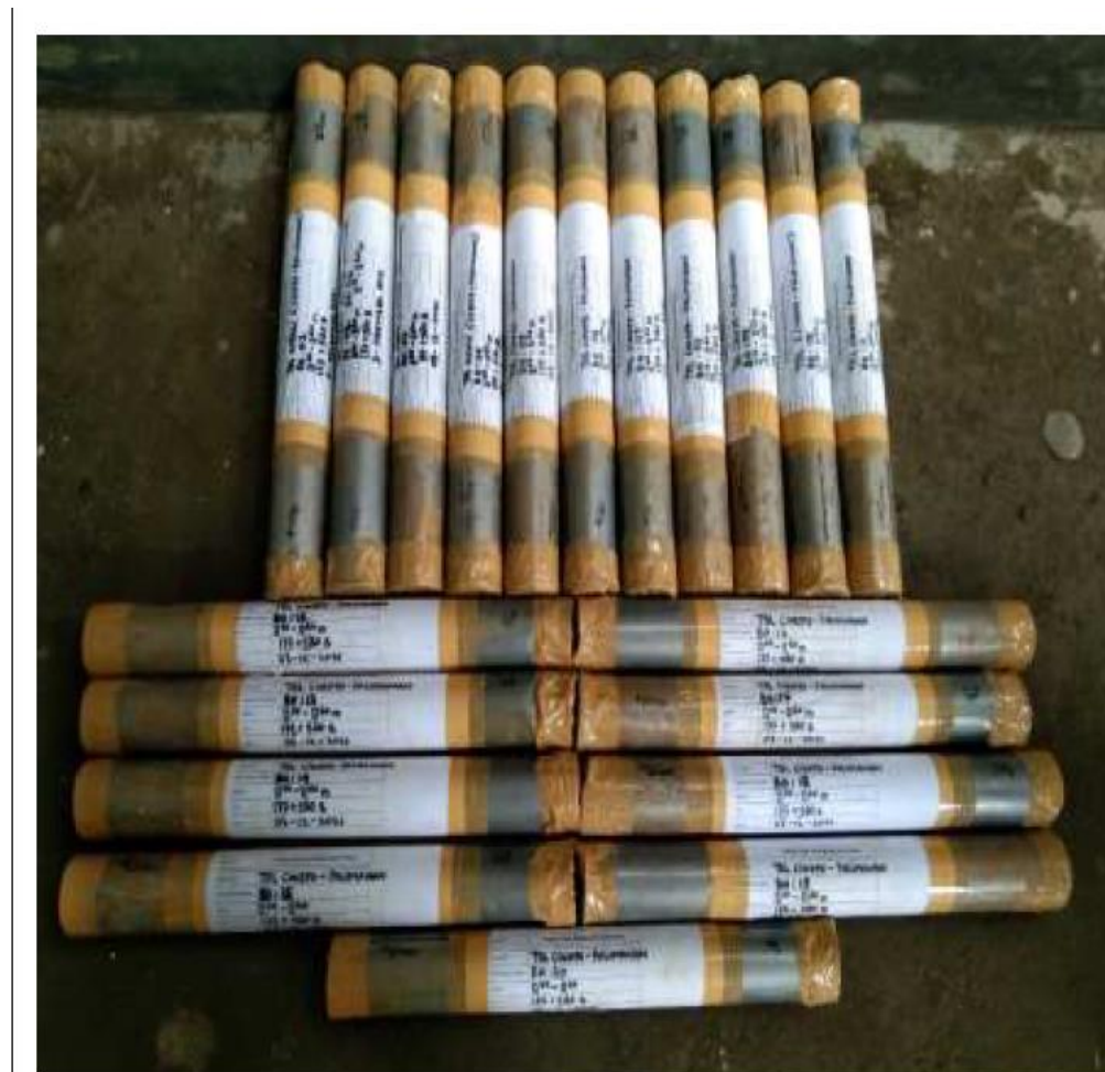
Figure 9. UDS in sealed tubing.
