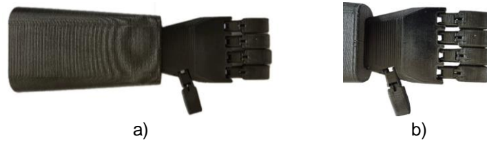
Figure 5. Transradial prosthesis prototype.
