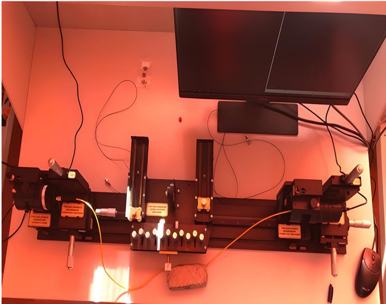
Figure 15. Study of the internal structure of a deformed optical cable.
