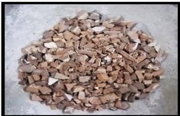
Figure 1. Porcelain Tile Particles Size Used in Concrete Mix.
