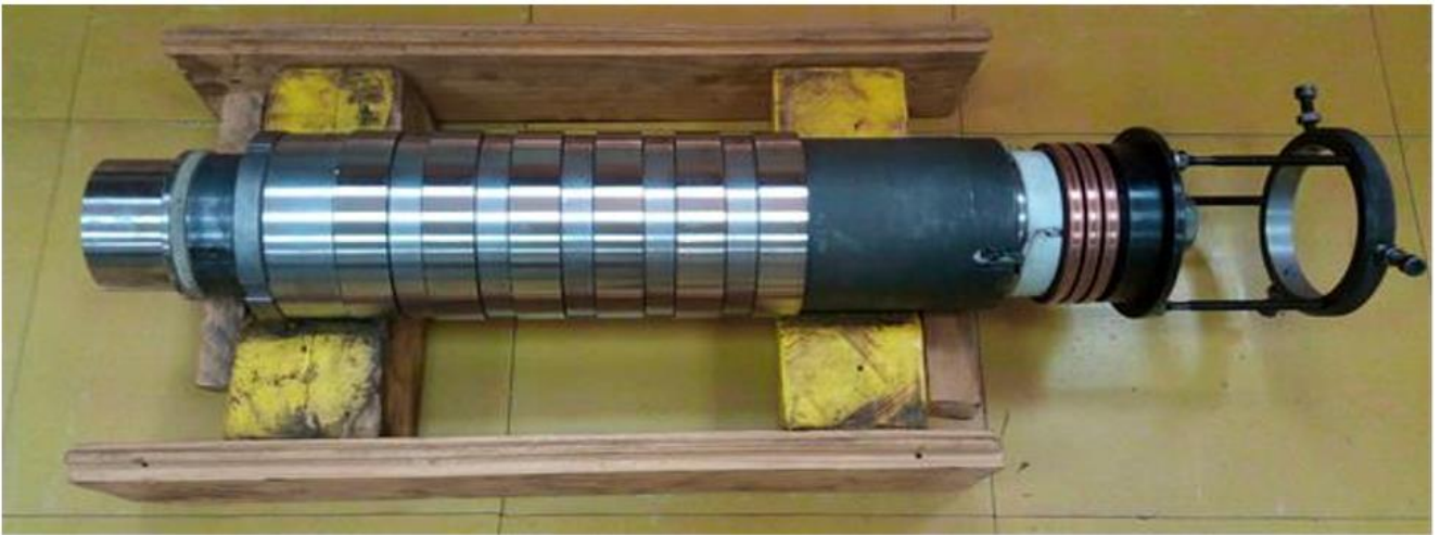
Figure 2. Special aid for the investigation of the average temperature in the cutting process during turning.
