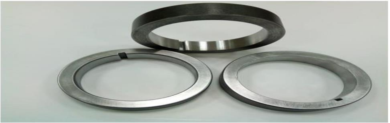
Figure 1. Rings of material C 65 (DIN), with hardness 65 \pm 2 HRC.
