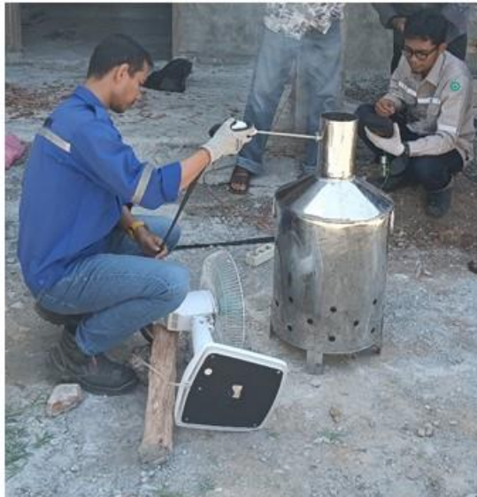
Figure 3. Emission test using Garden Incinerator for combustion and generic emission analyzer to monitor exhaust gas emissions.
