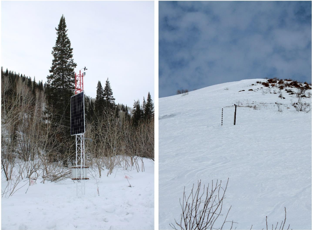
Figure 22. Base station and snow-temperature rod in an avalanche-prone area of the East Kazakhstan Region.
