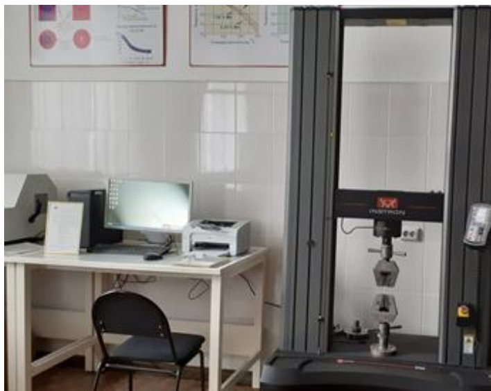
Figure 10. Electromechanical testing machine INSTRON 5980.
