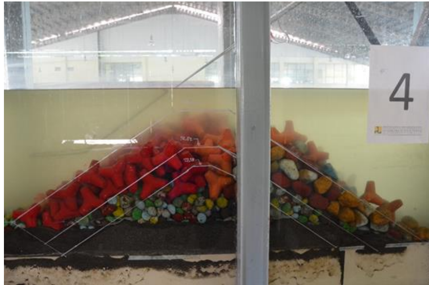
Figure 4. A rubble mound breakwater model with a 1:1.5 slope and a tetrapod main protective layer under a 0.70 m water level.
