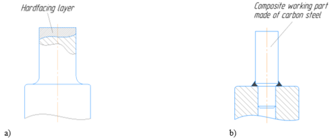
Figure 2. Methods for restoring busbar punching tools: a – restoration by hardfacing; b – composite tool design.
