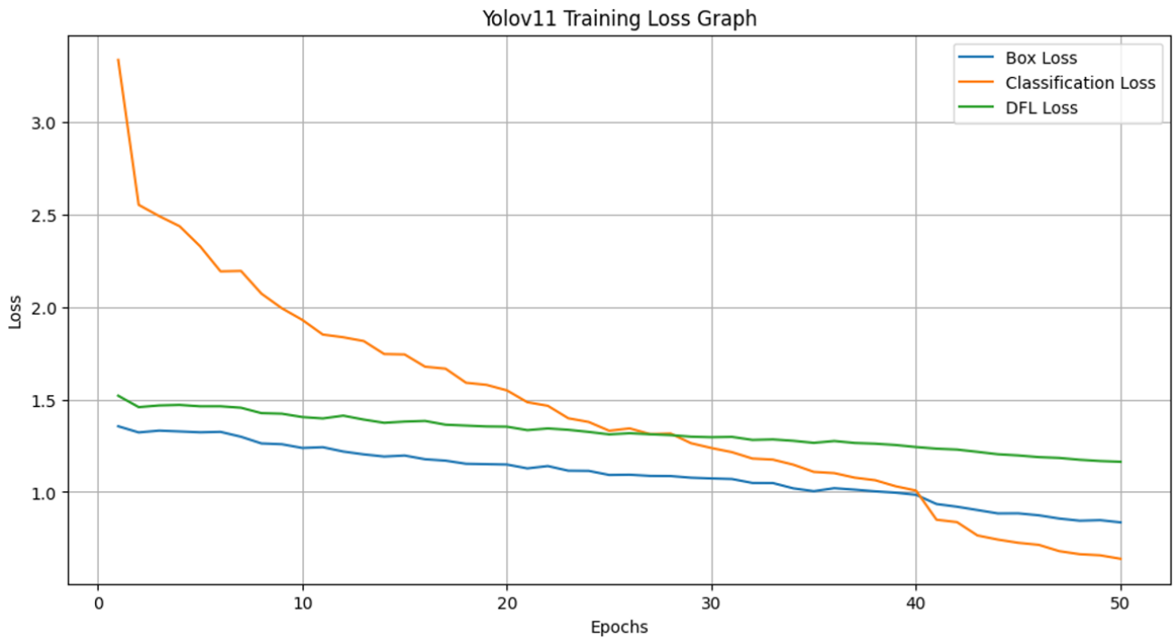
Figure 15. Training loss curves of YOLOv11 model.
