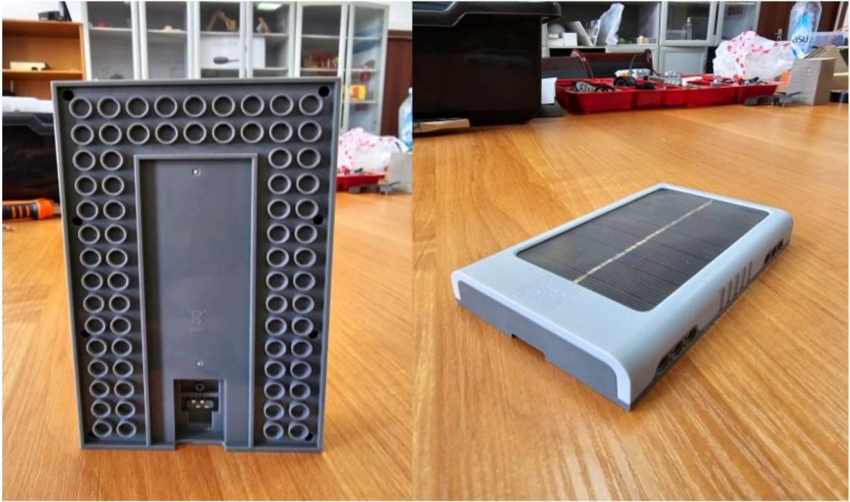
Figure 1. Solar panel in Lego EV3.
