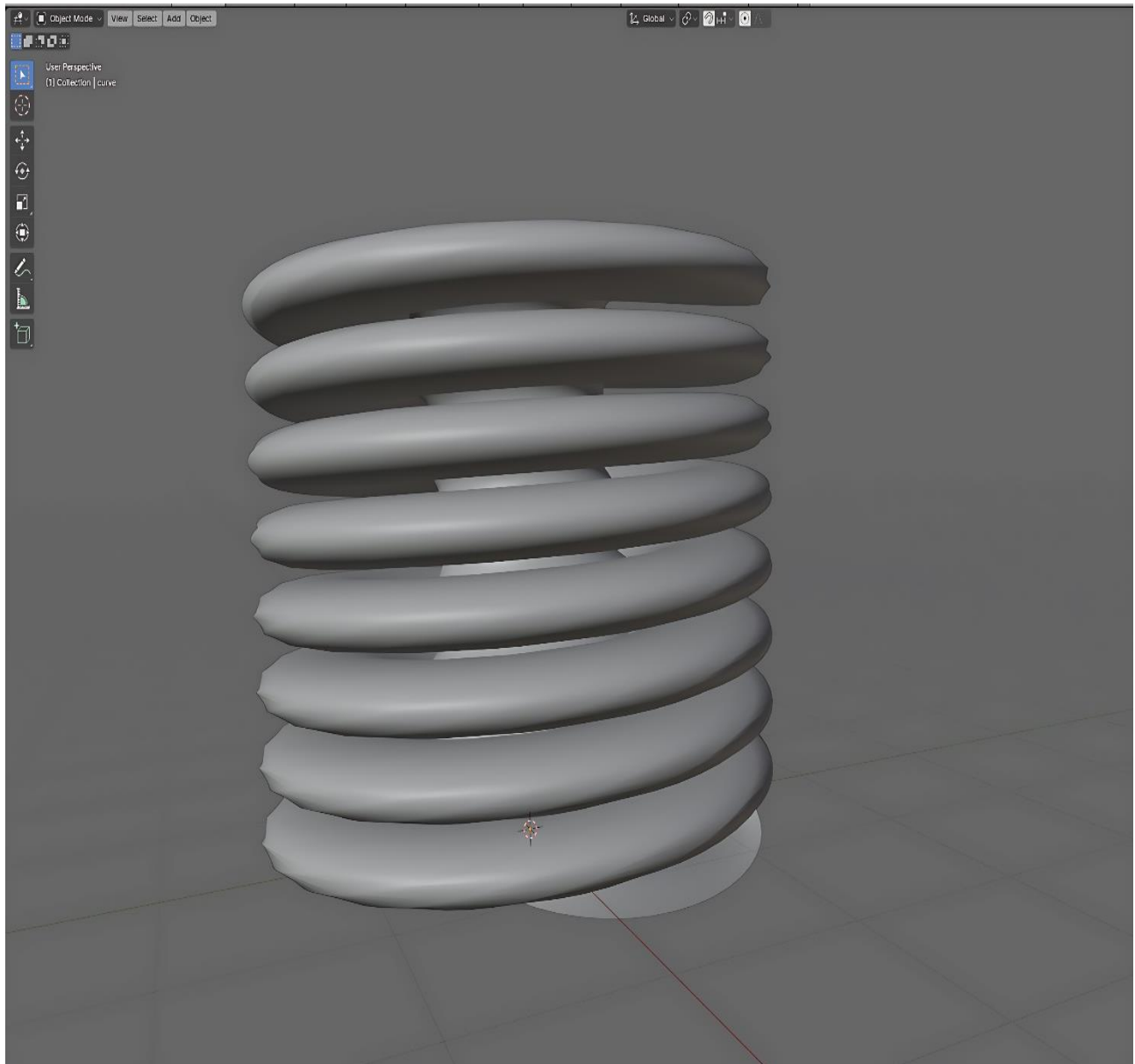
Figure 7. Using an array for a tank part.
