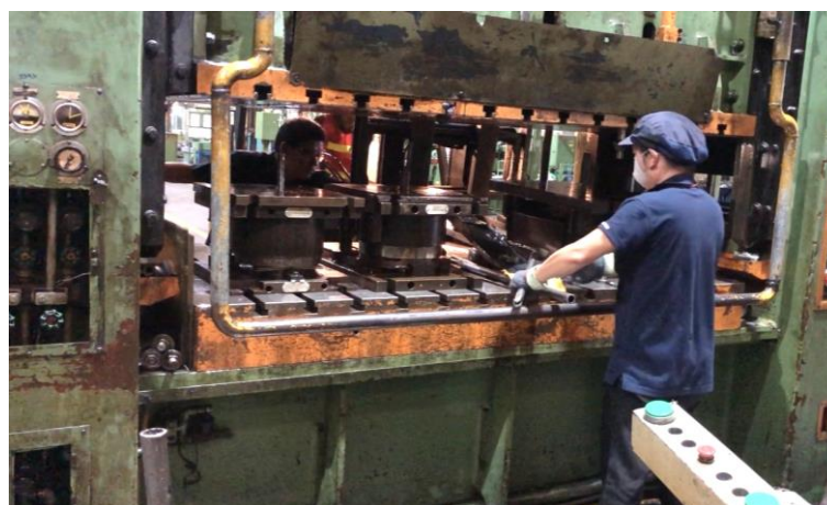
Figure 7. Adjusting the position of the die to align with the cushion holes.
