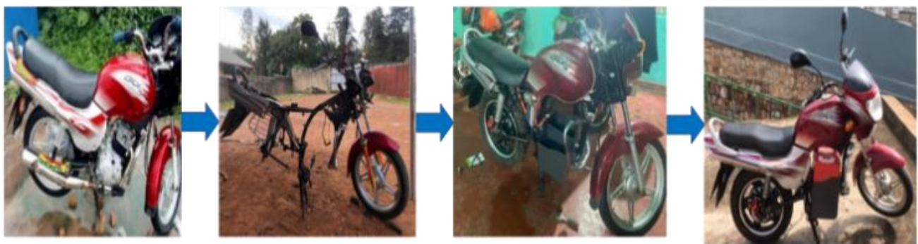
Figure 1. Retrofitting process: From original petrol-drive to full retrofitted at REM workshops.
