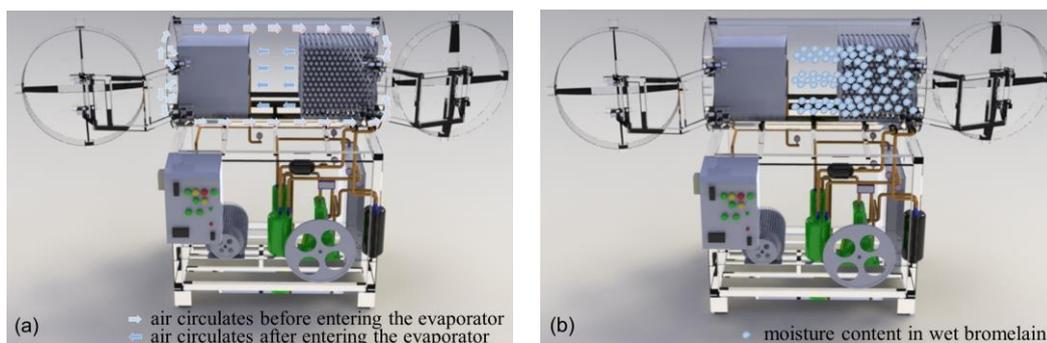
**Figure 3.** Freeze dryer consist of two processes: (a) the air blast freezing process and (b) the freeze drying process.
