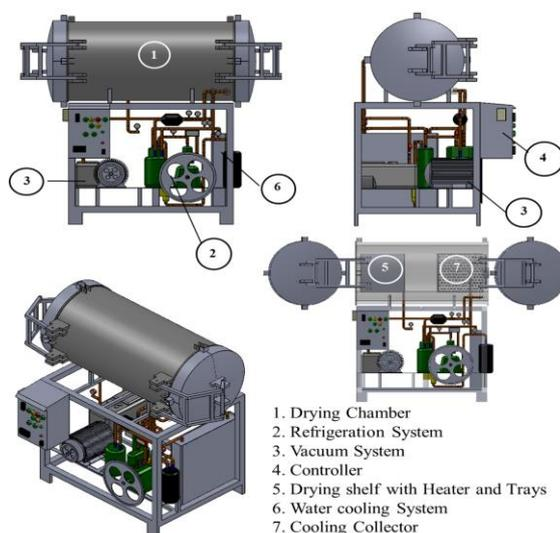
**Figure 1.** In-house freeze dryer with the vapor-compression refrigeration and water cooling systems.
