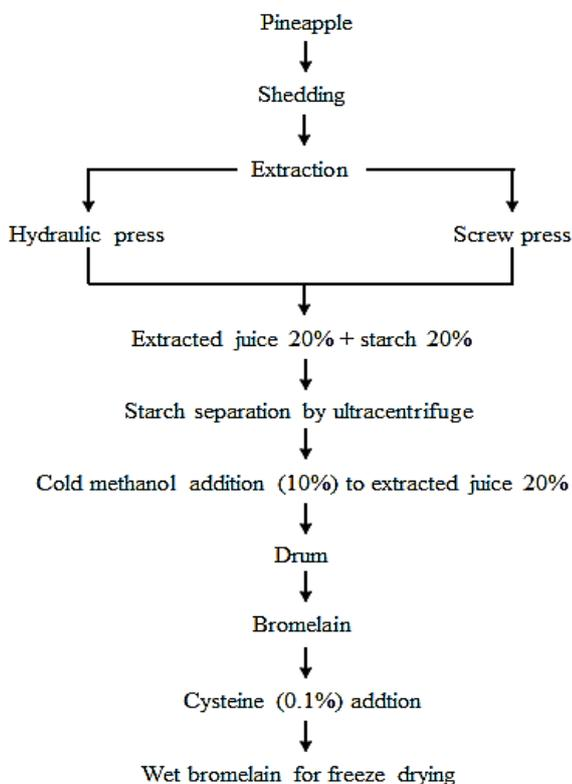
**Figure 4.** Crude enzyme process for bromelain extraction.
