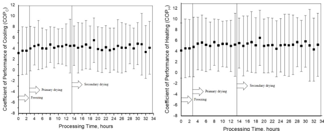
**Figure 8.** Evolution of coefficient of performance during cooling and heating operations.
