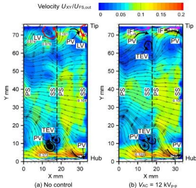
**Figure 10.** Velocity distributions at the exit of the linear turbine cascade,  $Re = 1.4 \times 10^4$  [2].
