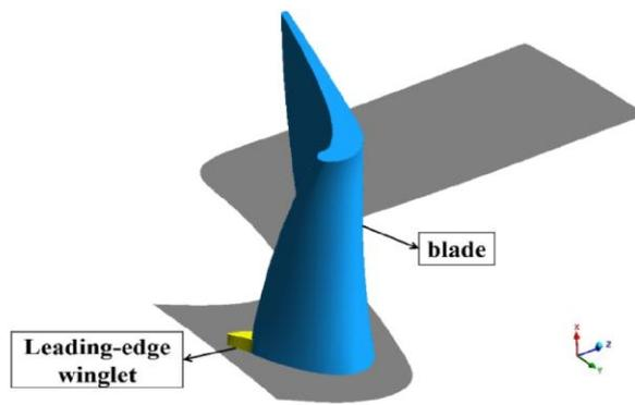
**Figure 3.** Geometric definition of the leading edge winglet.
