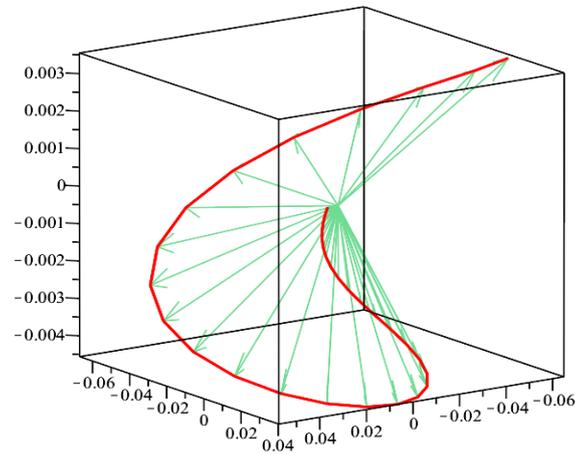
**Figure 5.** Linear acceleration  $a_{O_2}$  of the origin  $O_2$  of the moving coordinate system  $O_2X_2Y_2Z_2$  for 36 positions of the RRRRT manipulator.
