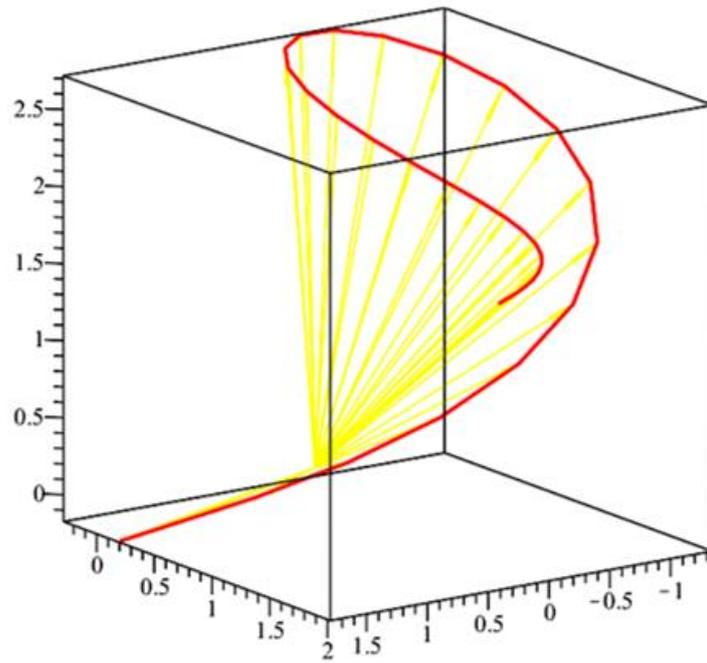
**Figure 2.** Trajectory of point P for 36 positions of the manipulator RRRRT relative to the base coordinate system  $O_0X_0Y_0Z_0$ .
