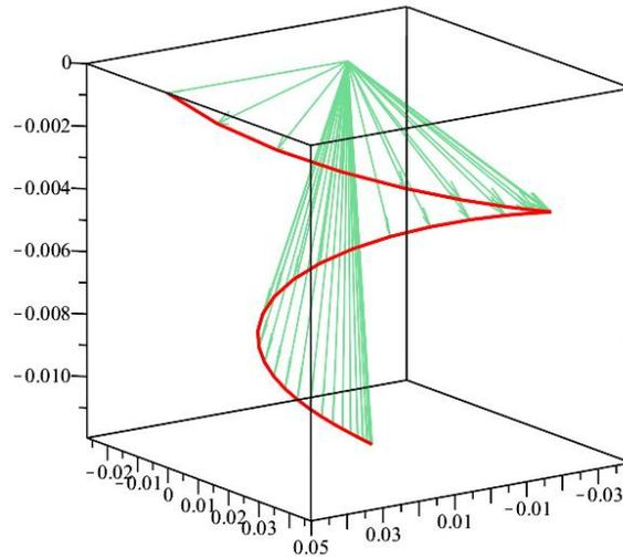
**Figure 4.** Angular acceleration  $\varepsilon_3$  of link 3 for 36 positions of the manipulator RRRRT.
