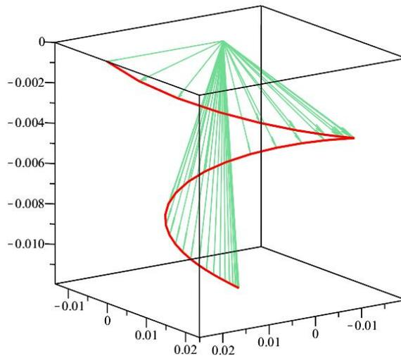
**Figure 3.** Angular acceleration  $\varepsilon_2$  of link 2 for 36 positions of the manipulator RRRRT.
