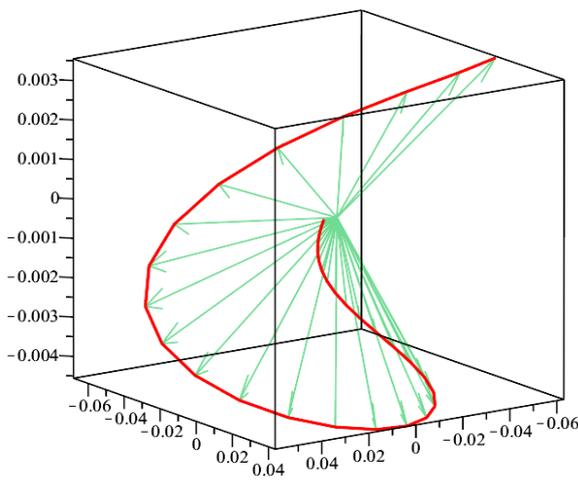
**Figure 6.** Linear acceleration  $a_{O_3}$  of the origin  $O_3$  of the moving coordinate system  $O_3X_3Y_3Z_3$  for 36 positions of the RRT manipulator.
