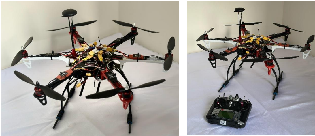
a) Hexacopter Structural Configuration and Electronic Components b) Hexacopter Pre-Flight System Readiness and Remote Control Interface
