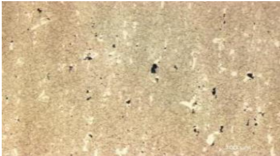
Figure 10. Optical microscopic structure of the cross-section of fusing layer ( \times 200 , Nital etching).
