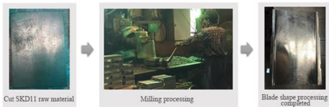
Figure 1. Processing sequence of STD11 rolled steel.
