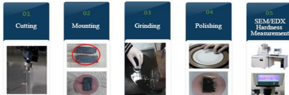
Figure 6. Cutting of surface-spray coated STD11 steel and tissue observation, and the process of fabricating test samples for hardness measurement.
