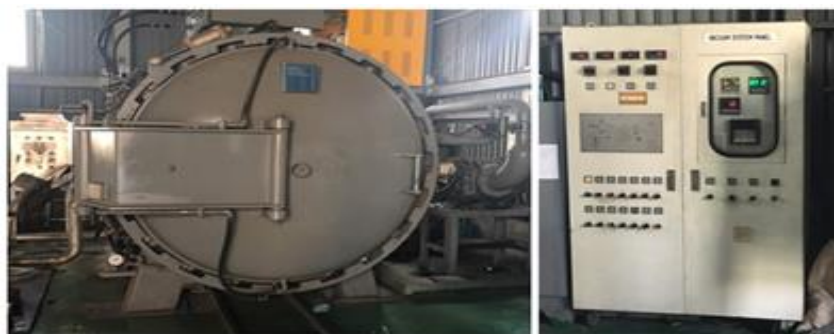
Figure 2. Vacuum heat treatment furnace and controller.
