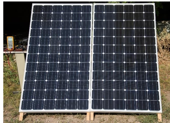
c) Segment of a photovoltaic system consisting of two solar panels
